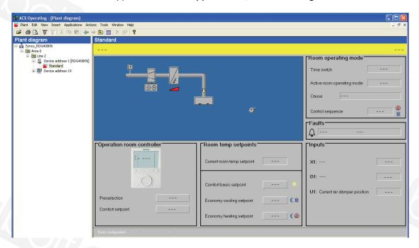
ACS provides standard plant diagrams for RDG KNX thermostats, which depend on the configuration as follows:
