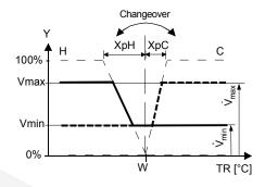
T[°C] Room temperature Room temperature setpoint Control command "Actuator" HqX Proportional band "Heating" XpC Proportional band "Cooling" Vmin Min. limitation for output Max. limitation for output
