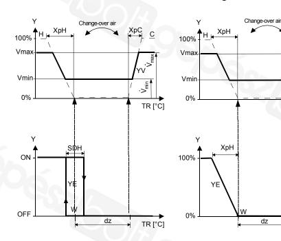
Without a valid bus signal for changeover air, the air volume is only increased for cooling:
