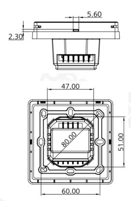
ARG800.1 single mounting frame for RDF800KN/NF
