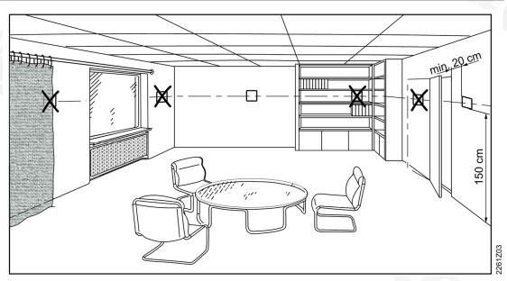
The device is designed for wall mounting and flush mounting.
