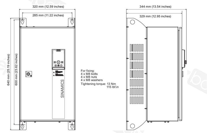
Figure 3-4 Dimensions and drill pattern, PM230 FSD (22.0 - 30.0 kW)
