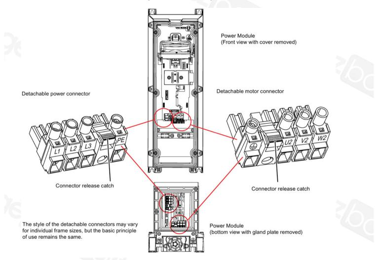
Figure 4-1 SINAMICS PM230 FSA to FSC power connections
