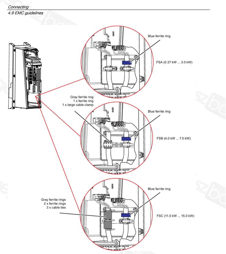
Figure 4-11 Fitting ferrite rings to motor and mains supply cables
