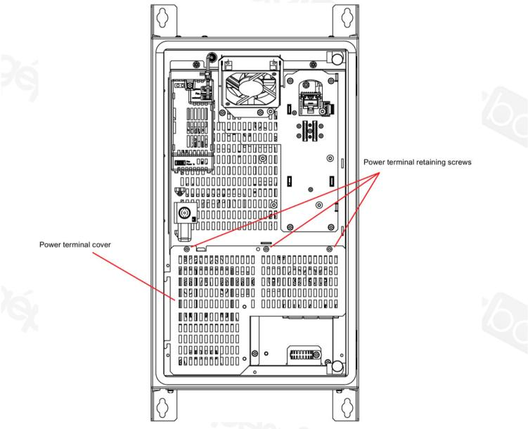
Figure 4-2 SINAMICS PM230 FSD to FSF Terminal Cover
