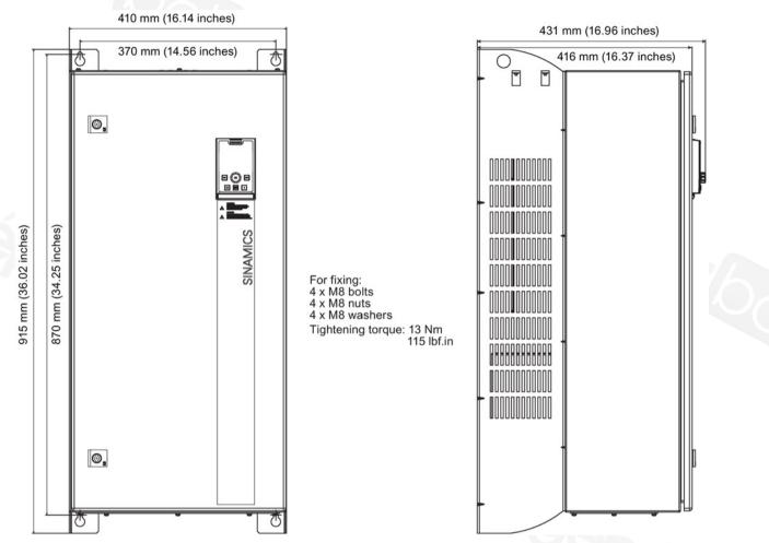
Figure 3-6 Dimensions and drill pattern, PM230 FSF (55.0 - 90.0 kW)
