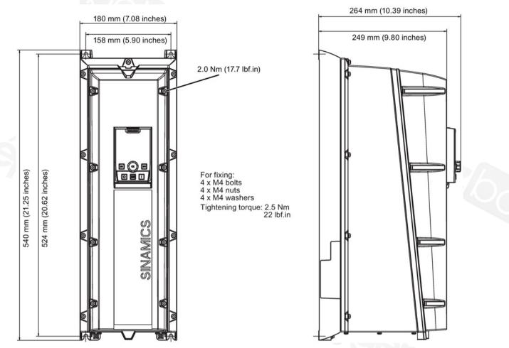
Figure 3-2 Dimensions and drill pattern, PM230 FSB (4.0 - 7.5 kW)
