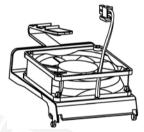
Figure 5-10 Replacement internal fan module FSA to FSC
