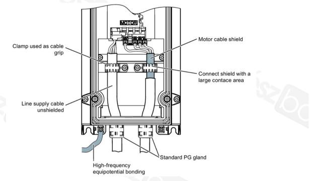
Figure 4-9 Power Module shielding, FSA ... FSC
