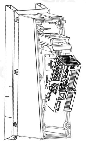
Figure 3-7 Fitting CU to PM
