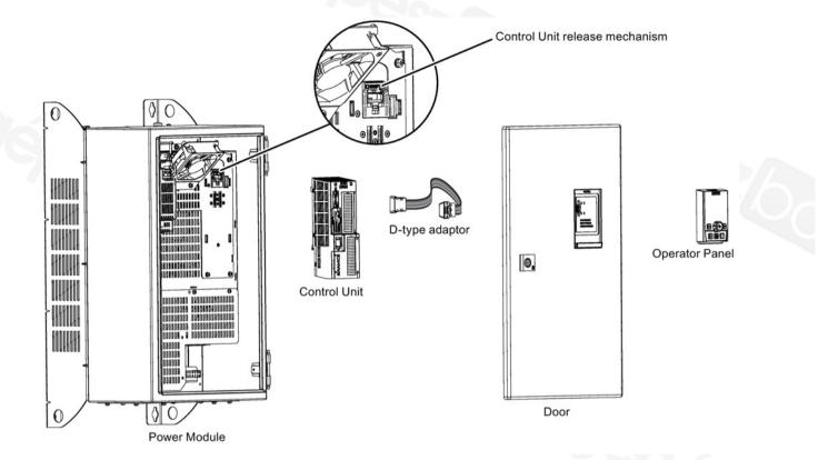
Figure 3-10 Fitting CU to PM230 FSD to FSF
