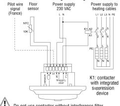
Do not use contactor without interference filter.
